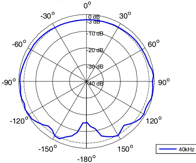
Typical Equivalent Noise Pressure Curve
